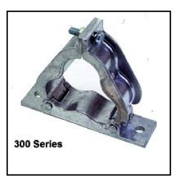
Trefoil clamps are used to hold 3 types of cable or conductor together on shelves, ocean beds in trenches or where the application is required. Clamps can be fixed with a single internal (500 series) or double external (300 Series) arrangement. Trefoil clamps are cast and manufactured from bicon alluminium alloy.
